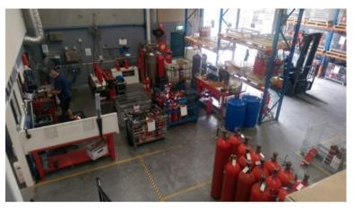
Prior to undertaking any Hydro-static test, all cylinders are subject to a full external and internal examination to ensure that any corrosion or other defects are within the specifications outlined in the Australian Standards. Any cylinders not meeting those specifications cannot be tested.
